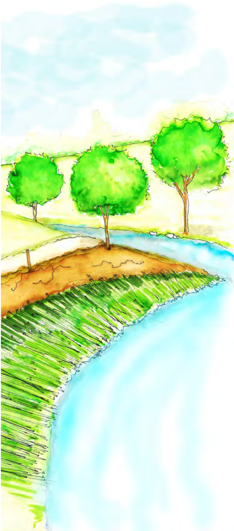
Fig 3.3 Sketch of a revetment with cuttings alongside a little stream.
