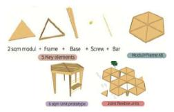
Fig. 5 - Components of singular modules and their composition into joinable units. Authors' work
