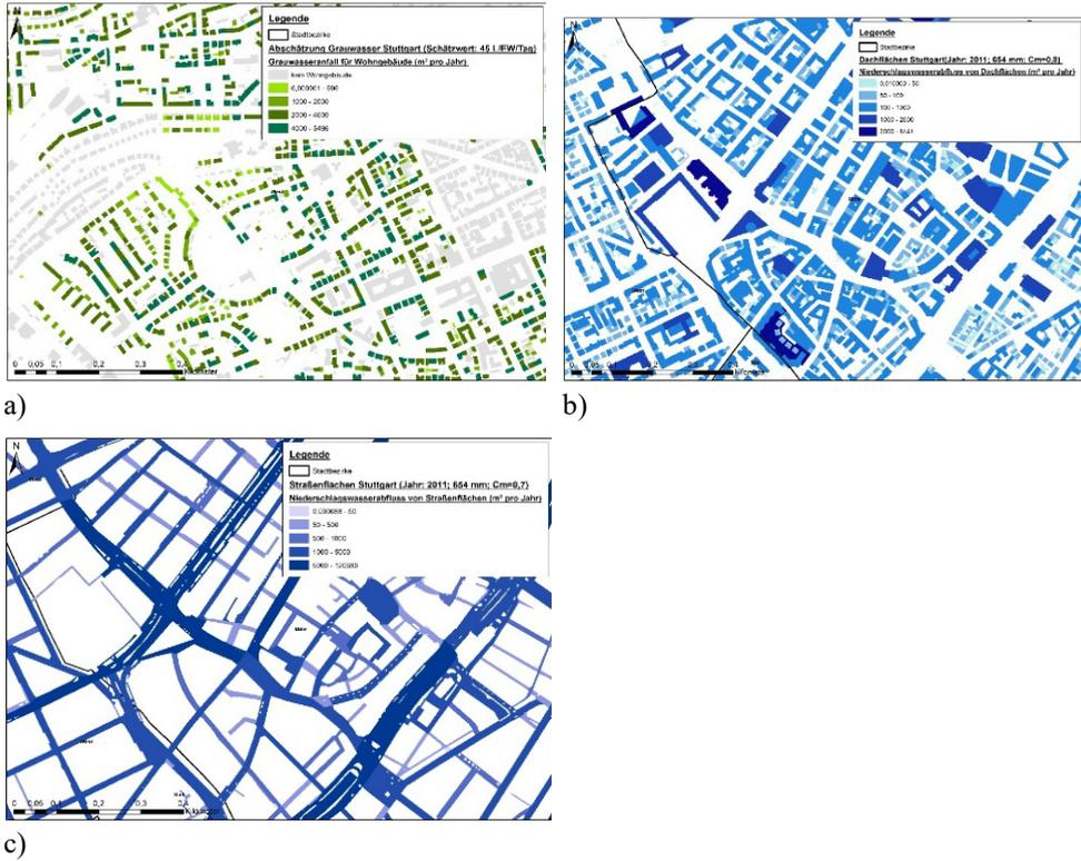
**Fig. 1:** Water harvest from grey water, roof drain and street drain summed up for the year 2011: a) grey water, b) roof runoff, c) street runoff
